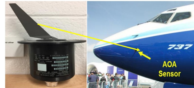
FIGURE 2: AOA SENSOR FIGURE 3: AOA LOCATION ON A BOEING 737
